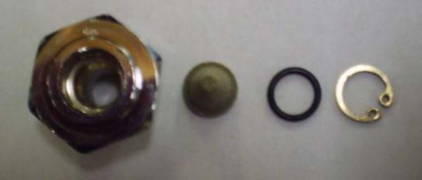
Remove Piston Cap and HP spring, HP Seat, Piston, Spacing Shims, HP Seat and O-Rings, LP and HP plugs
