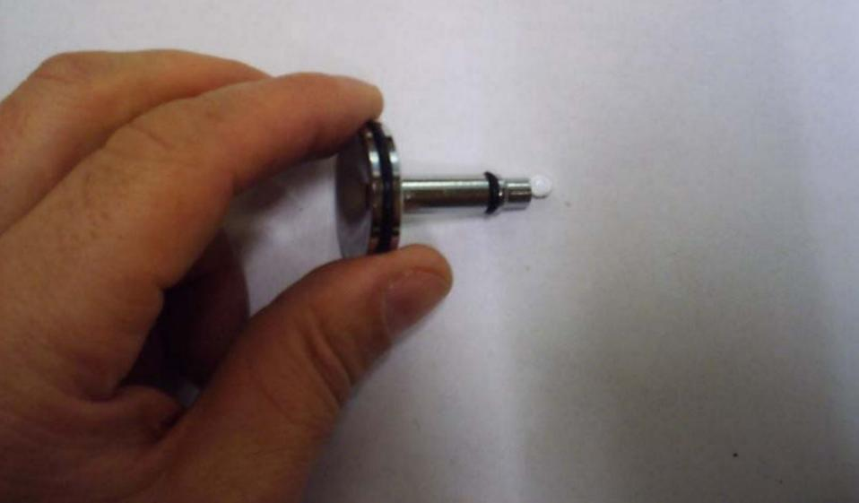
Insert piston through spacing shim, HP spring and into the regulator body
