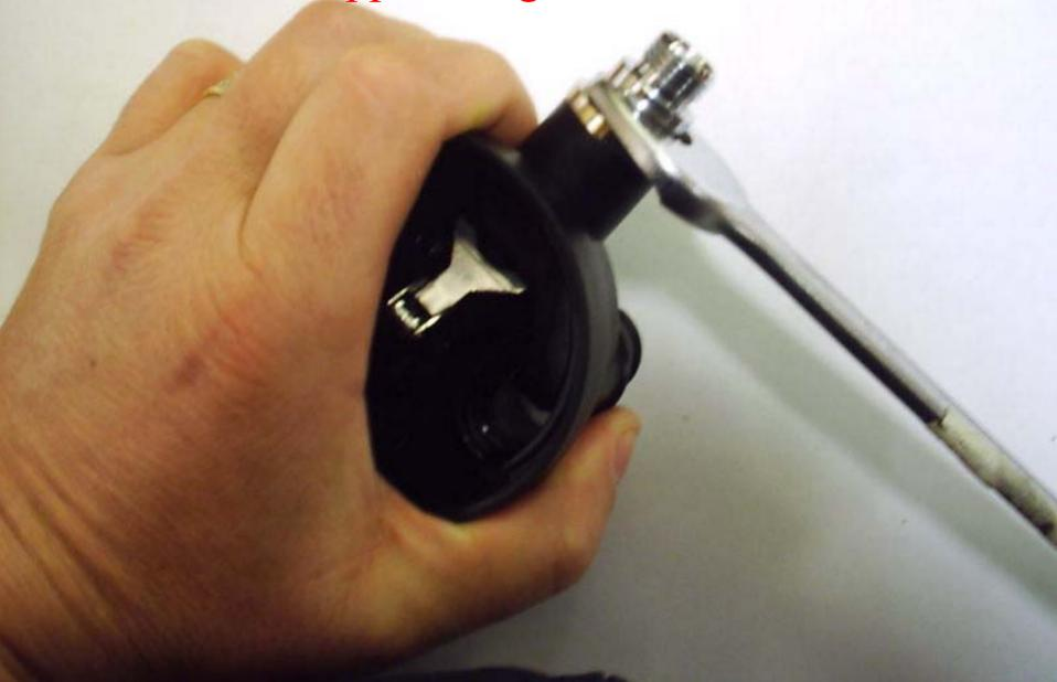
Remove Lever Arm by pushing seat carrier and pulling lever arm
